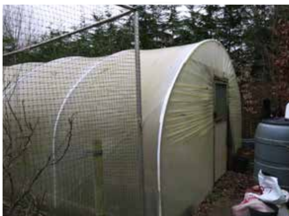
Fig. 3.2 Fragmentation of PE with exposure to UV in a cool temperate climate at 61.6 °North; (a) standard PE sheeting, (b) PE sheeting with UV stabilizer added, for horticultural use. © Peter Kershaw
